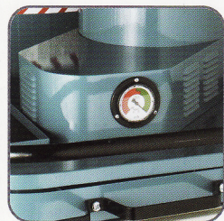
Vacuum meter (manometer)
